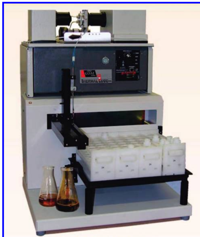
Figure 1. COAT FTIR system designed for the automated analysis of oils and lubricants.
